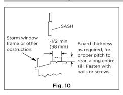
Add wood as shown in Fig. 10, or remove storm window before air conditioner is installed.
