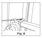
6. To secure lower sash in place, attach right angle sash lock with 3/4" (19mm) or 1/2" (12.7mm) screw as shown (Fig. 8).
